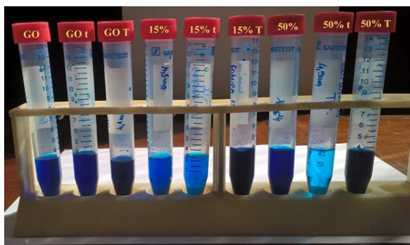
Figure 2. Appearance of samples after adsorption of methylene-blue
